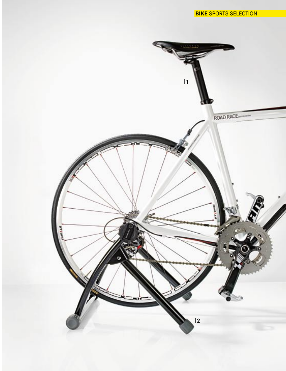
|2 PROP STAND Aluminium/stainless steel. Simple, universal attachment to rear wheel quick-release mechanism. Space-saving, fold-away design. Load capacity of up to approx. 90 kg. B6 799 5766
