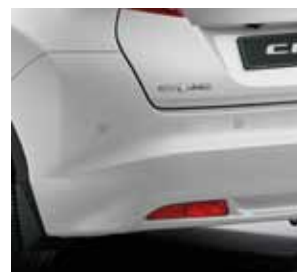
13 Rear Parking Sensors
