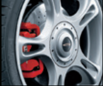
16-inch sport brake with perforated and grooved front brake discs
